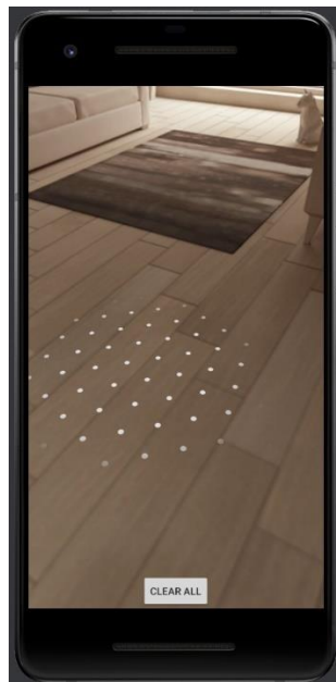
Figure 9 – Establishing a Plane Using ARCore (Image is taken within a virtual environment)
